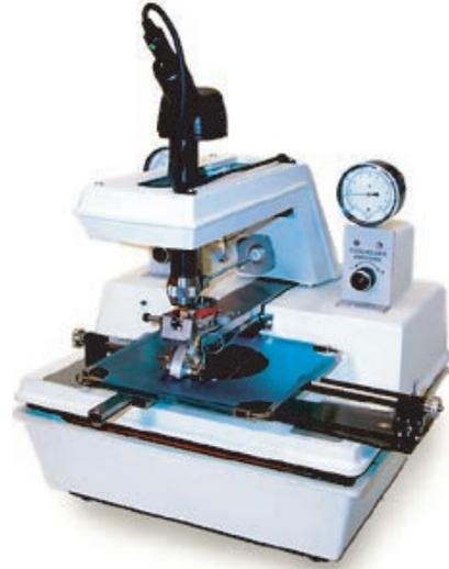
The scribe line guides the break. It is a single crack across the wafer that causes the wafer to break into strips, or the strip to break into dice. The LSD-110, like the LSD-100, uses beam bending to induce tensile strain lateral to the scribe line. The break mechanism extends across the entire scribe line.
