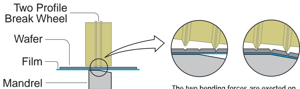
The two bending forces are exerted on the separation grids between the dice.
