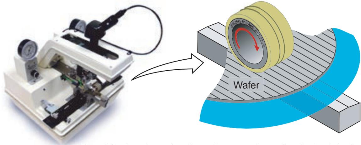
Two of the three beam-bending points come from a break wheel that has raised tracks formed around the circumference.
